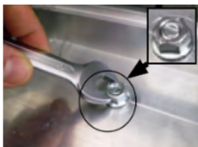
Loosen the nuts on the inside face and leave the heads of the studs aligned to realise the profile
