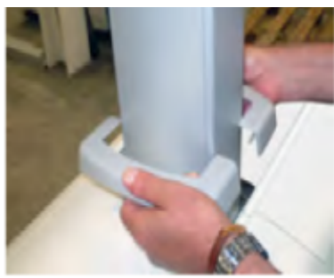
Separate the covers next to the suspension
