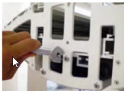
Remove the screws that fix the lower profile
