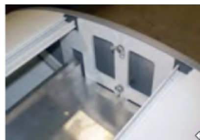
Extract the end covers by removing the wingnuts
